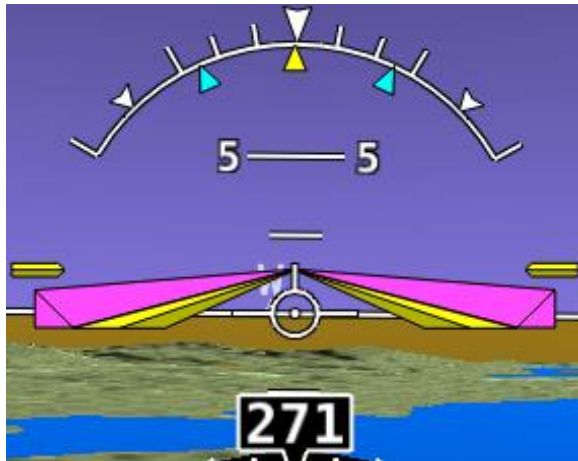
Figure 206 - Single Cue / Inverted-V with Autopilot Servos Engaged
