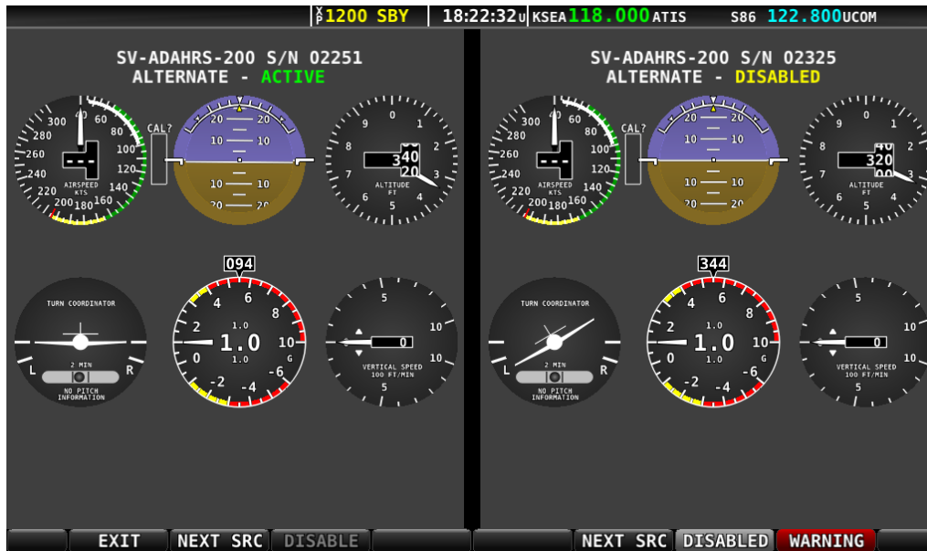
Figure 57 - ADAHRS Cross-Check Comparison – six-pack
