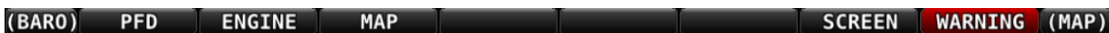
Figure 226 - Message Notification Area above button 8 (2nd from right), showing a Warning Notification
