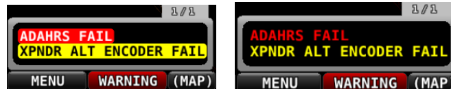
Figure 228–Unacknowledged (left) and Acknowledged (right) Alarms
