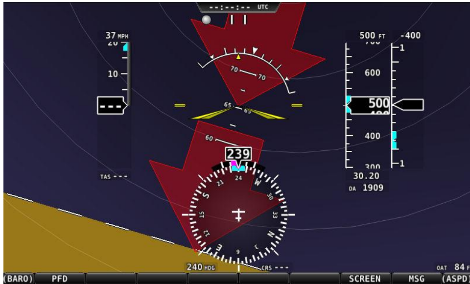
Figure 51—Extreme Pitch Warning Indicator Arrows
