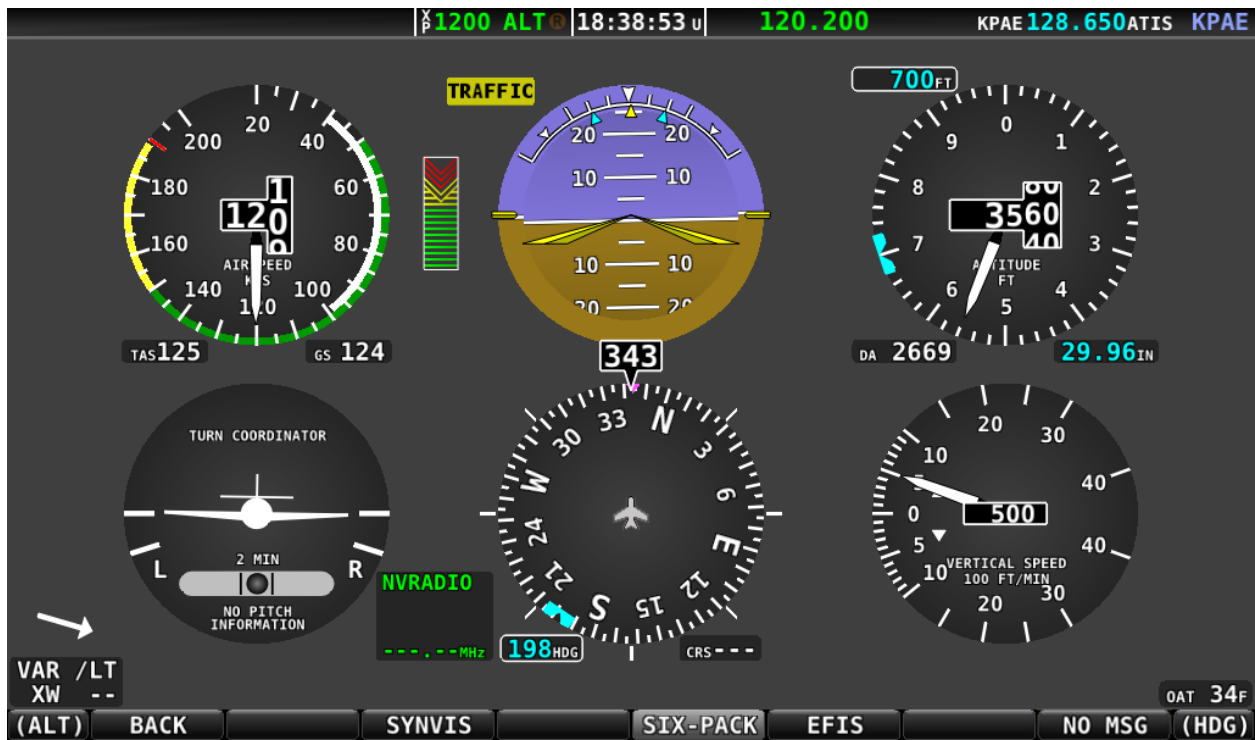
Figure 53 - Analog PFD without Synthetic Vision
