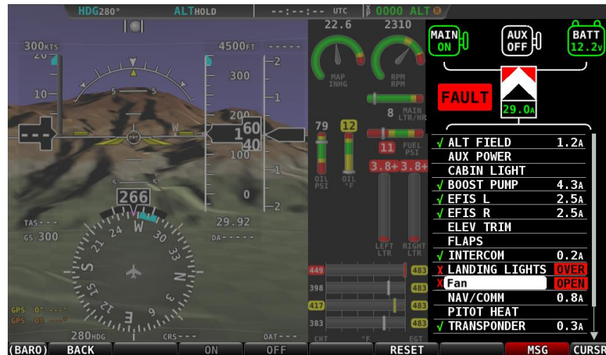
Figure 73 - VP-X Page with Fault
