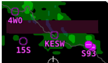
Figure 154 - Missing NEXAD Data Blocks
