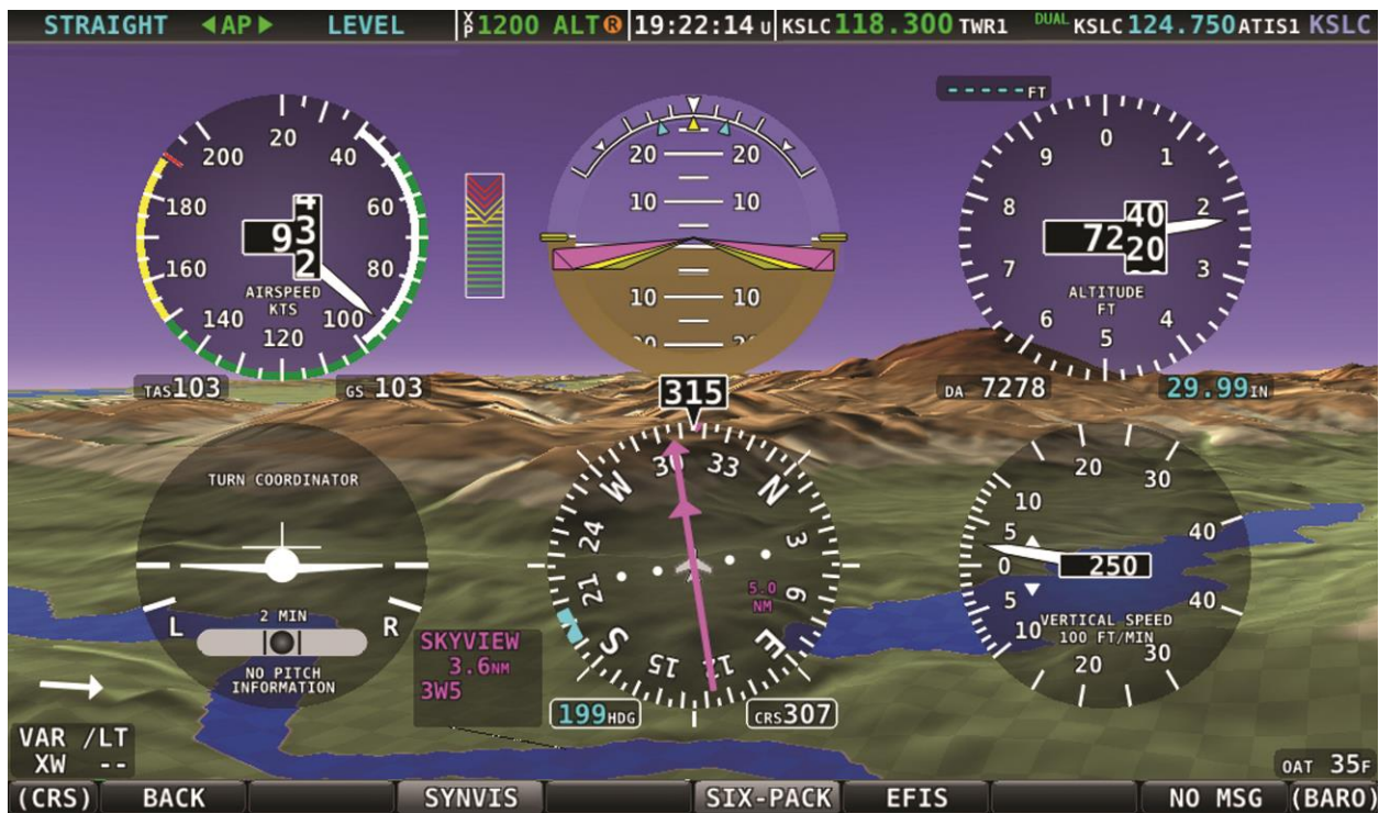
Figure 52 - Analog PFD with Synthetic Vision
