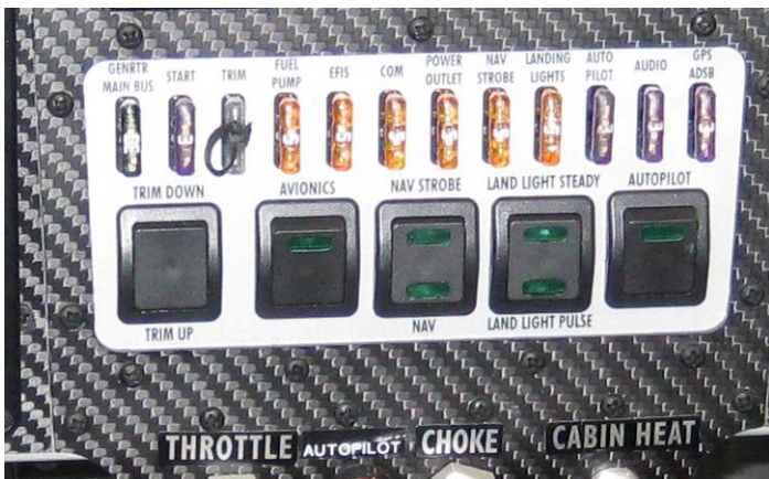
SKYVIEW/G3X FUSE PANEL
